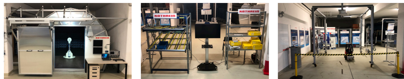
Anechoic chamber for automated transponder measurements and test areas for eKanBan and gate solutions
