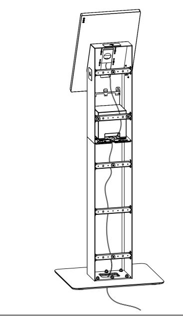
Step 8: Carefully reattach the two backplates.
