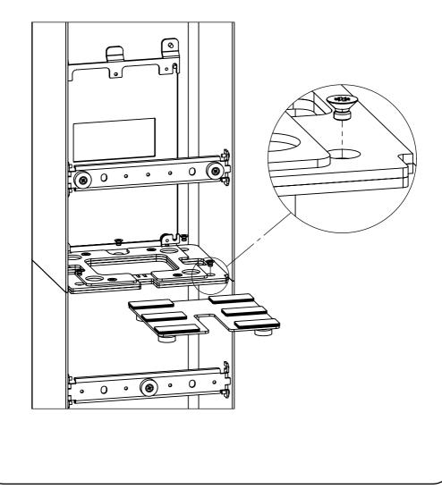
**Step 4:** Remove the protective paper from the Velcro. Position the printer as far forward as possible, and then press the printer down onto the self-adhesive Velcro.
