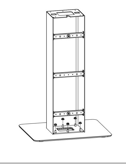
**Step 3:** Remove the printer plate by lifting it up, and then attach the top and bottom modules using the five included M5x6 countersunk screws, tightening them securely.
