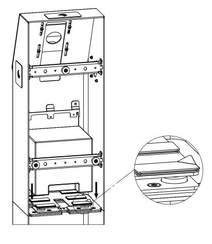
**Step 5:** Mount two of the included thumb screws to the top VESA holes on the screen and hook the screen onto the keyholes of the VESA plate. Then, attach the remaining two thumb screws to the bottom two holes on the screen and tighten them securely.
