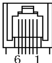
Fig.6.7-1 Schematic drawing of cash drawer interface
