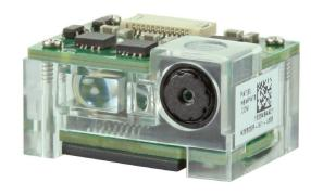
With its compact dimensions and integrated decoder, the N3680 2D imager makes it easier to incorporate enhanced performance scanning into your designs.
