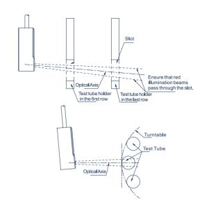
The product has anti-reflective characteristics, ensuring that scanning performance remains unaffected even when the optical axis is perpendicular to the barcode plane.
